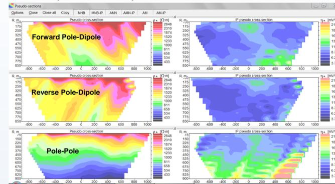
All resistivity and chargeability data contain some element of noise. The Pole-Dipole and Dipole-Dipole arrays are particularly susceptible to noise. The raw data below is plotted at the MN receiver electrodes.
